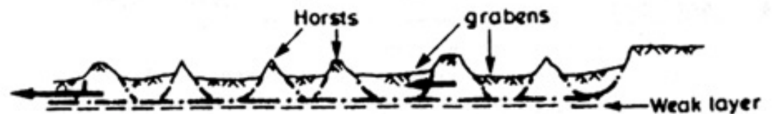
(f) Sudden spreading failures
