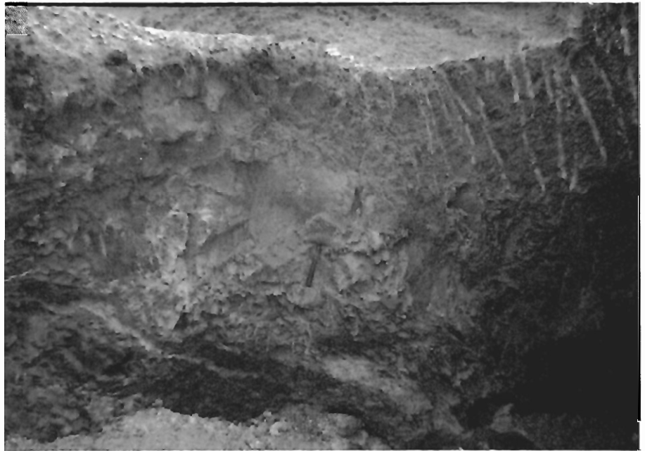
Fig. 1.8 Asbestos veins along small joints and shears, at Hero Shah, Malakand agency.
