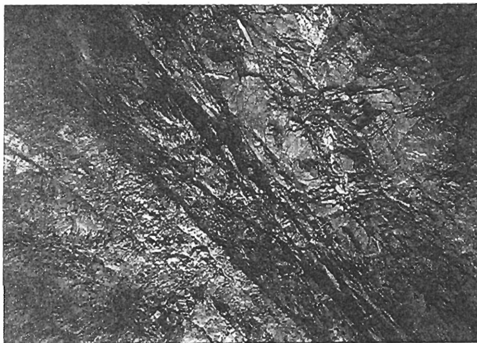
Photograph-3.12. Photomicrograph of Koga Syenites showing the veins of albite+ore and pyroxene+ore+albit. (Crossed nicols, magn.x25).
