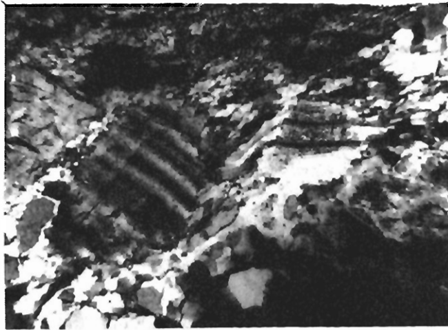
Plate-32. Photomicrograph showing kinked and corroded plagioclase grain indicating deformation, (Nicols crossed, Magni. x 25).
