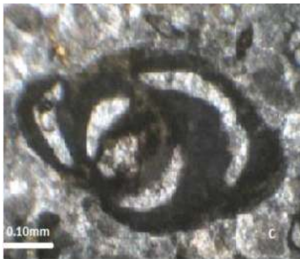
Fig. 13. Photomicrograph of microfacies of the Mishan Formation: a) Bioclast packstone ( Rotalia Viennoti ), b) Bioclast packstone, c) Bioclast wackestone, and d) Intraclast bioclastic wackestone.
