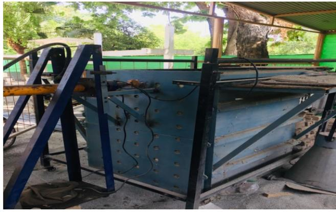
Fig. 5 Sand Box with Lateral Load Cell.
