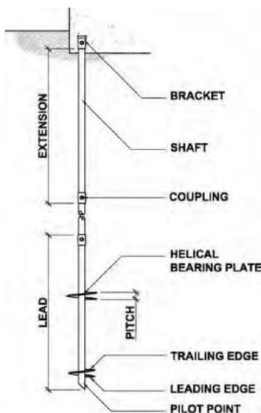
Fig. 1. Components of Helical Pile (Perko, 2009)
