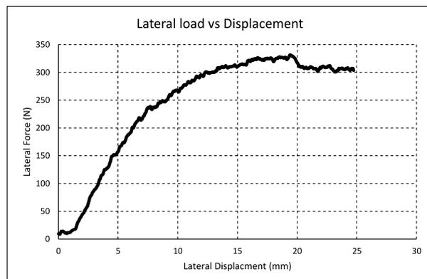
Fig. 17. Single Pile Single Helix Load vs Displacement.
