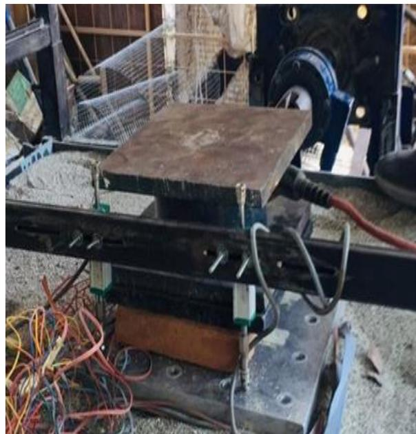
Fig. 13. Axial Load Cell.
