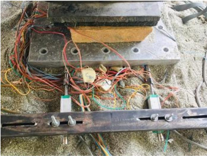
Fig. 14. LVDTs attached to Pile Raft
