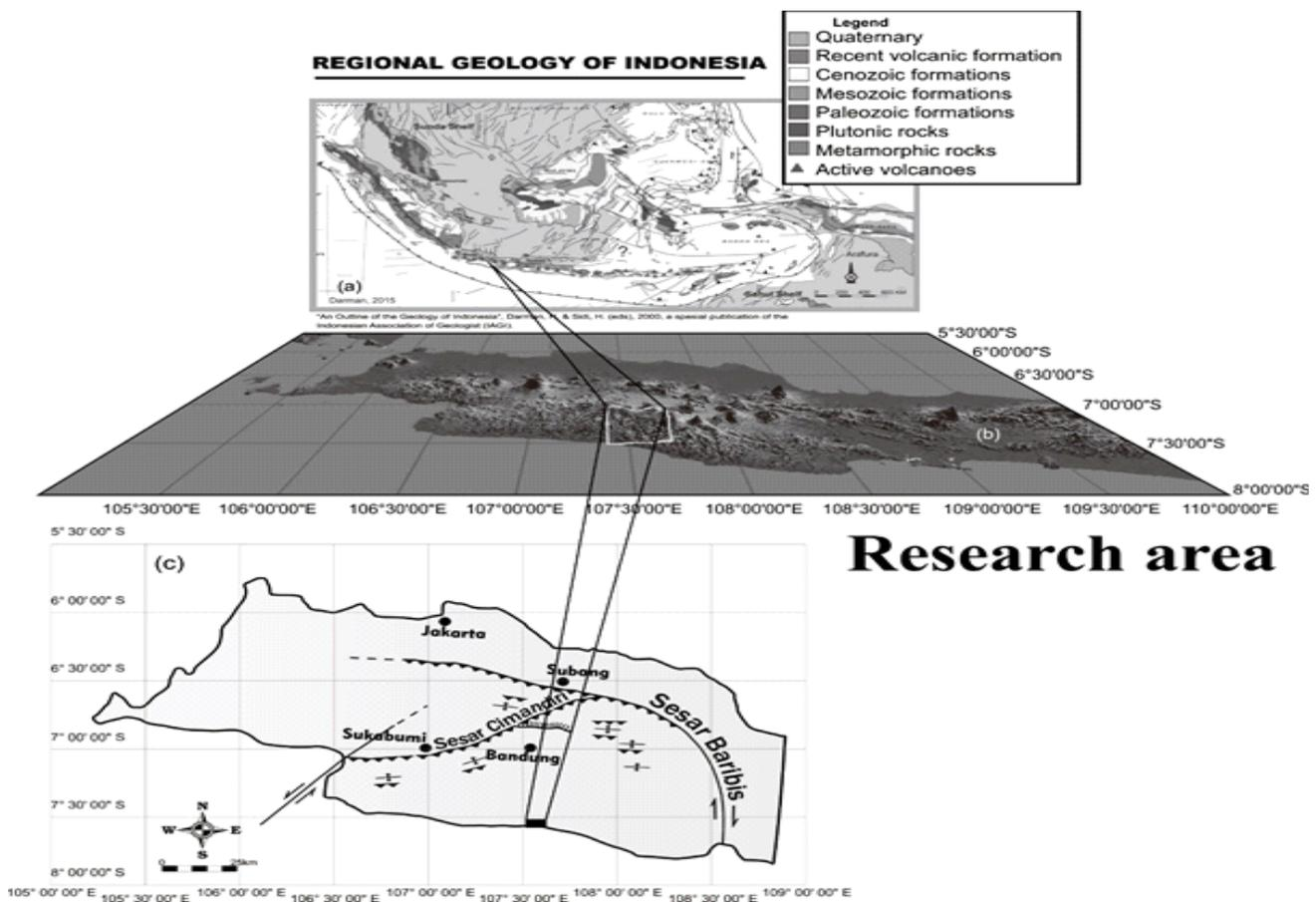
Fig. 1. (a) The regional geological setting of Indonesia; (b) the location of the research area in Cisewu regency, Southern Garut West Java Province; and (c) the major faults of West Java are the Baribis Fault, the Cimandiri Fault and Lembang Fault.
