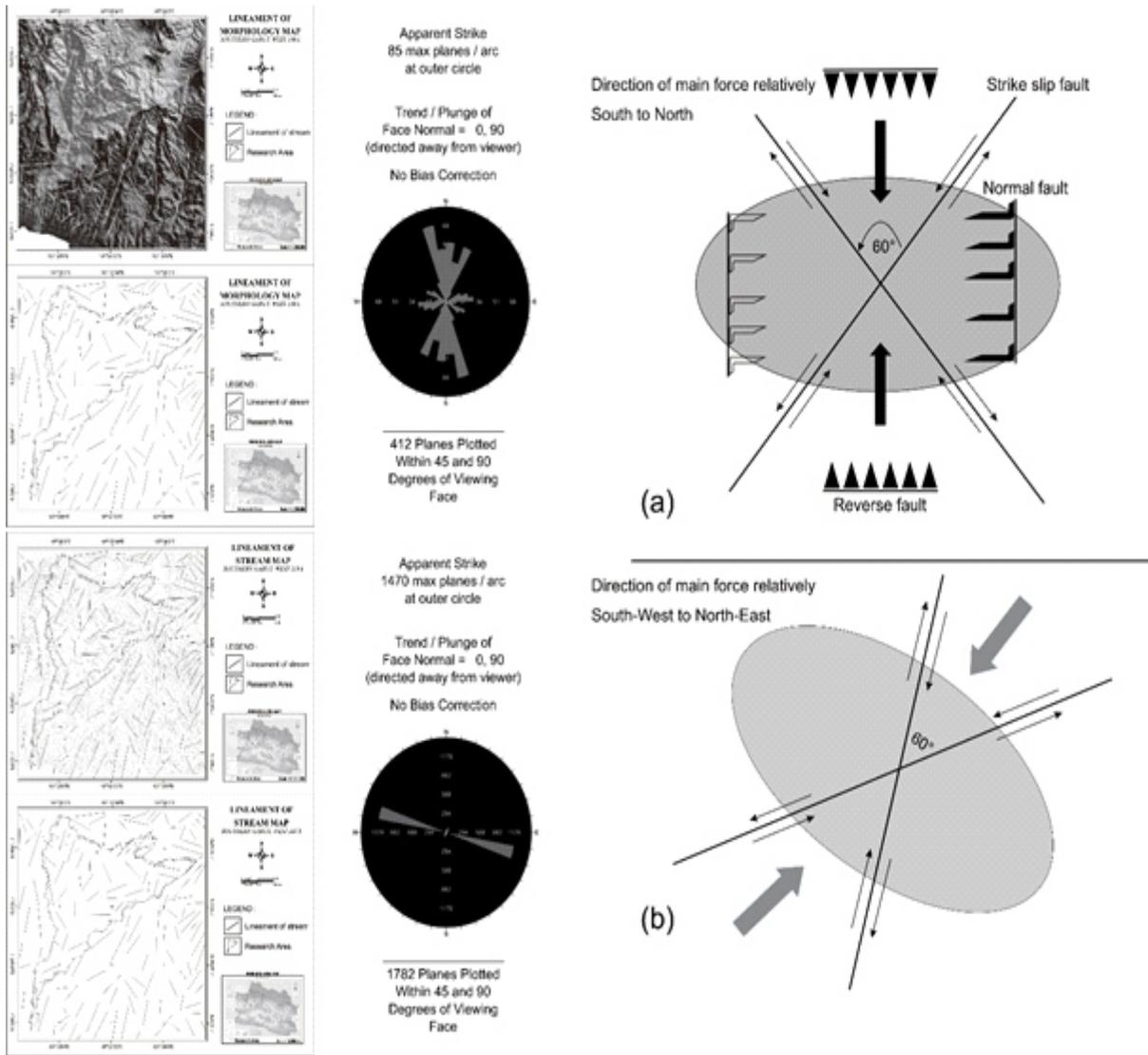
Fig. 3. The result of structural lineaments analysis showing a) a compression forces from South-North and b) a compression forces from SouthWest-NorthEast.
