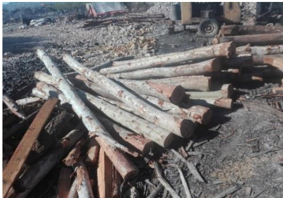
Plate 12. Eucalyptus is being used as Timber support in coal mines.
