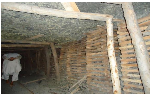
Plate 9. Poor roof supporting system in coal mines.
