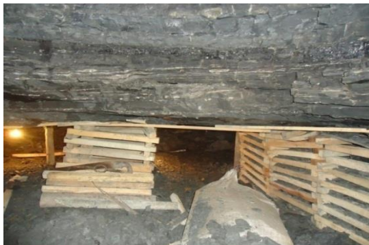
Plate 4 and 5. Field photograph representing use of Timber for support in Coal Mines.
