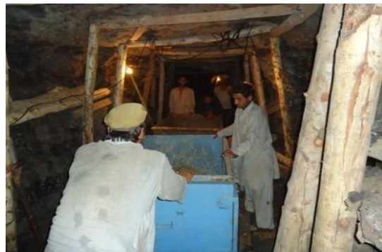
Plate 4 and 5. Field photograph representing use of Timber for support in Coal Mines.
