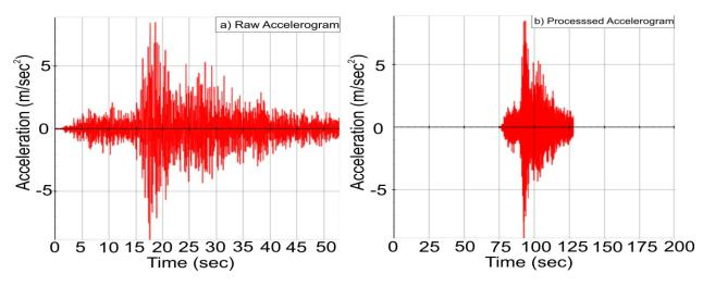
Fig. 5. Illustration of the filter and unfiltered profile.
