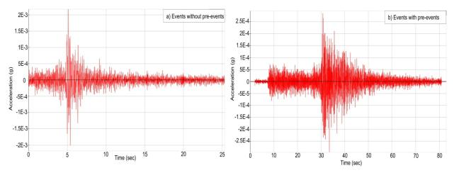
Fig.3. Example of raw data and Mean Removed Accelerogram.
