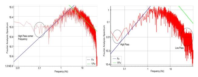
Fig. 4. Example of Acausal filtering shows High- and Low-cut pass frequencies with circles.
