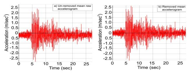
Fig. 2. Example of raw data and Mean Removed Accelerogram.
