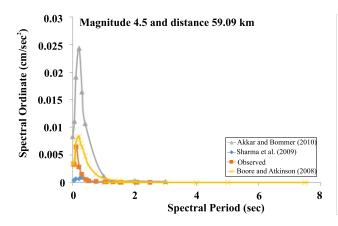
Fig. 6. (a) Graph showing the response spectra for the observed and calculated values.
