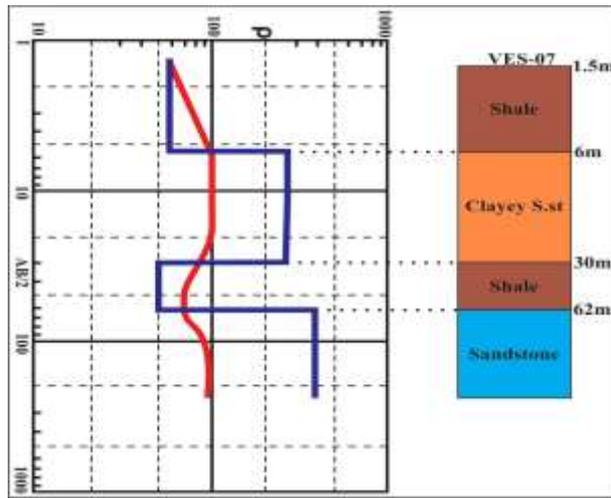
Fig. 2. Geoelectrical lithological section numerical modelled VES data of the study area using IPI2win.
