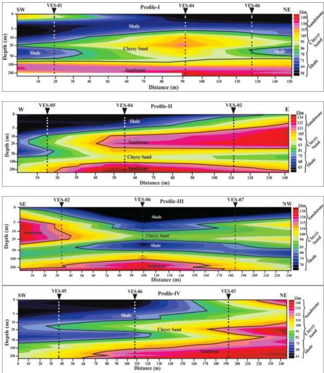
Fig. 3. Apparent resistivity Pseudo section of VES01 to VES07 stacked along P1-P4.
