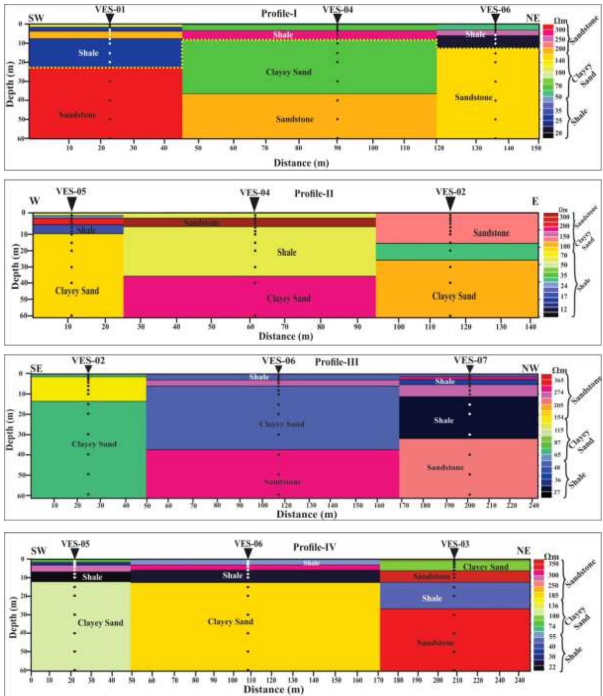
Fig. 4. Resistivity cross section of VES01 to VES07, stacked along P1-P4.
