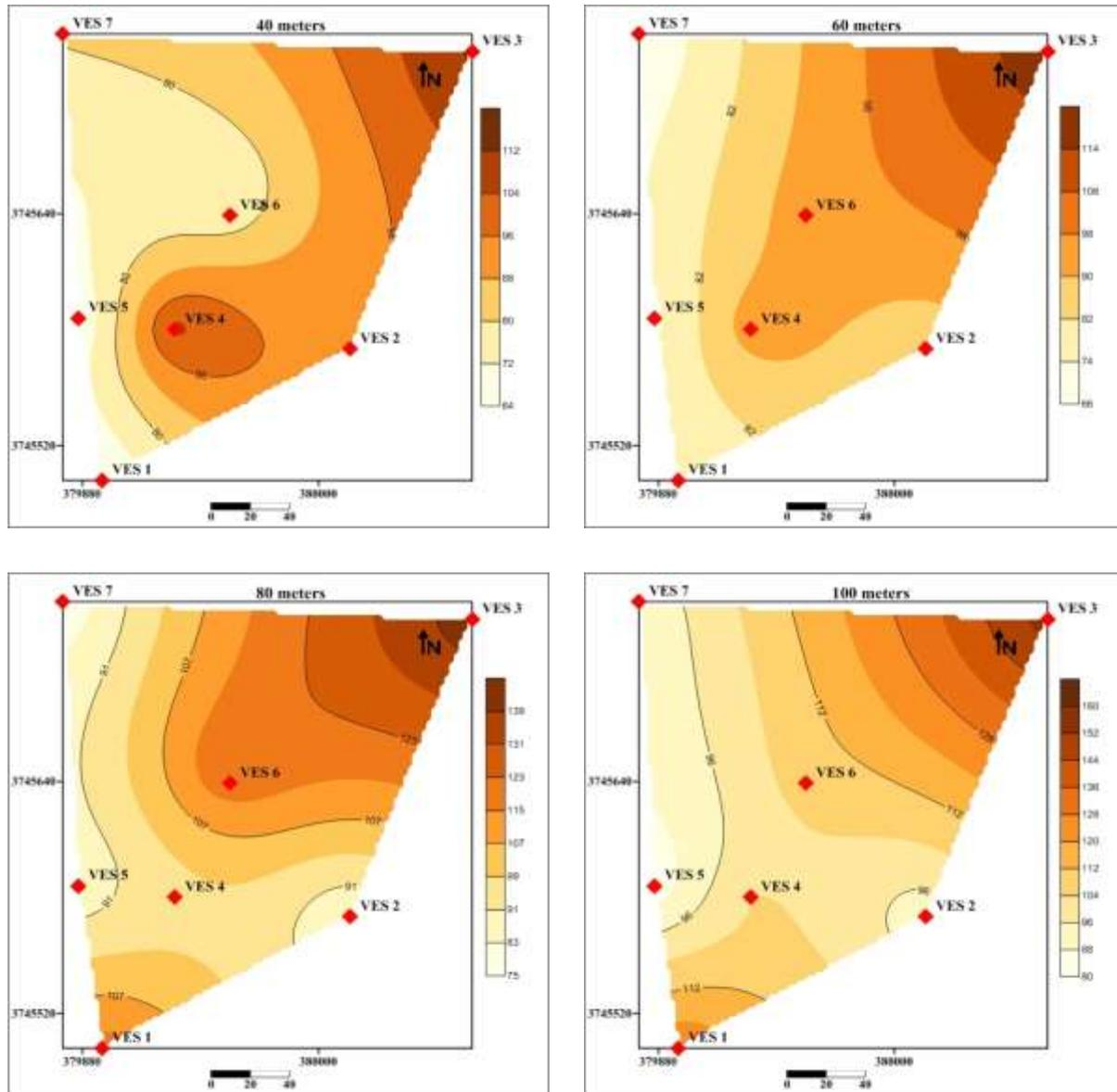
Fig. 6. Spatial distribution of apparent resistivity at (AB/2) 40 m, 60m , 80m and 100 m of the study area.
