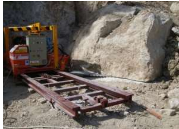
Fig. 6. Chain saw cutting (horizontal and vertical) (Rehman, 2010)
