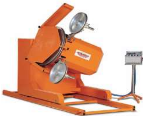
Fig. 3. Diamond wire saw machine (Rehman,
