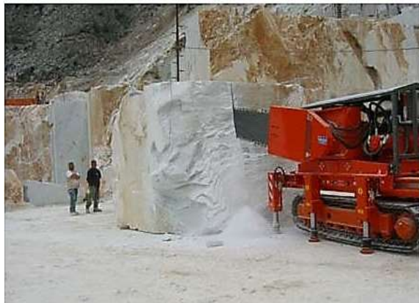
Fig. 6. Chain saw cutting (horizontal and vertical) (Rehman, 2010)
