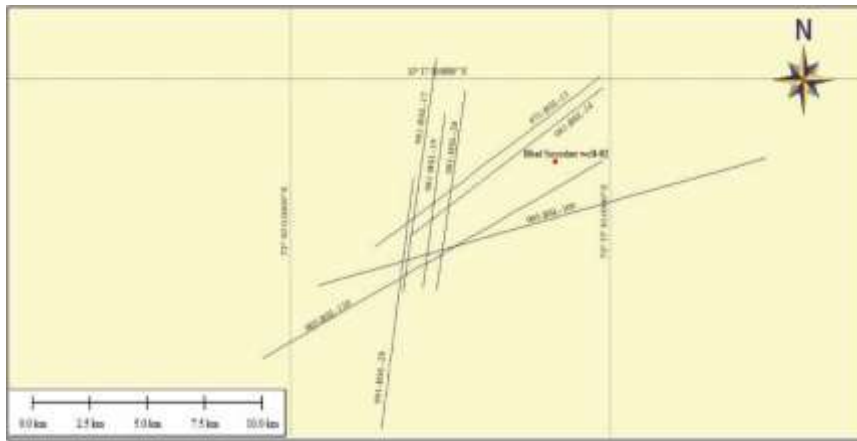
Fig. 2. Base map of the study area showing the location of seismic lines and Bhal Sayedan well-02.
