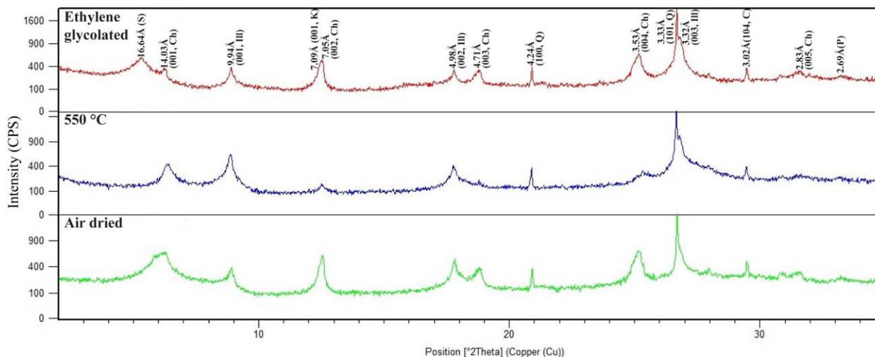
Fig. 6. XRD diffractogram of clay fraction of mudstone of the Malthanai formation, showing effects of different treatments on clay minerals.
