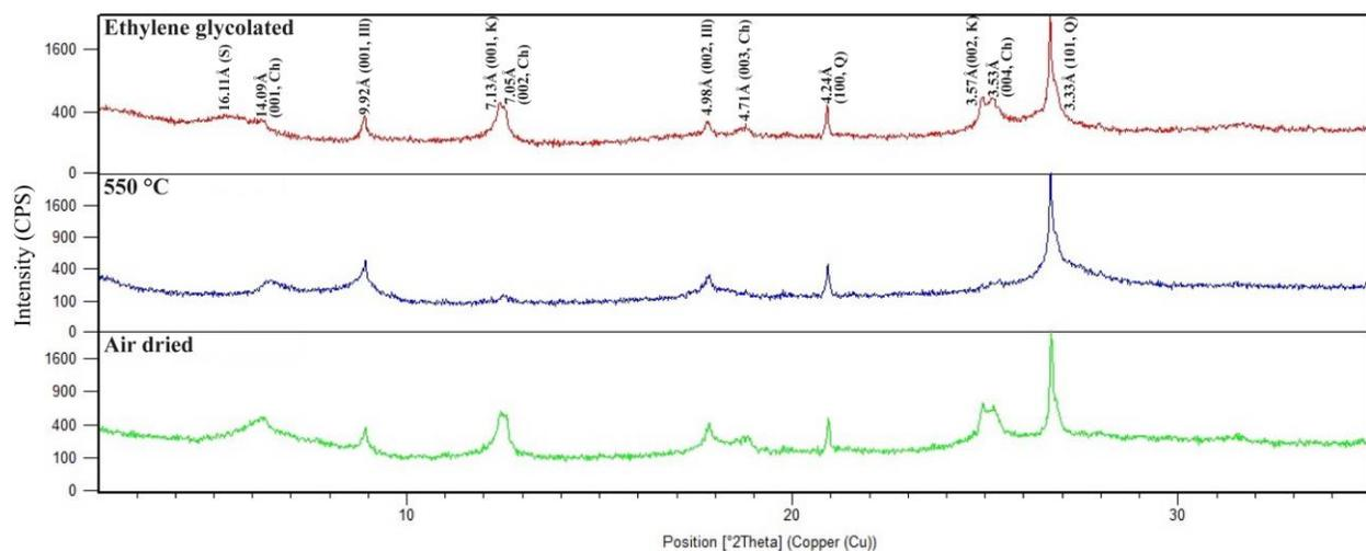
Fig. 5. X-Ray diffractogram of clay fraction of mudstone of the Dasht Murgha group, showing effects of different treatments on clay minerals.
