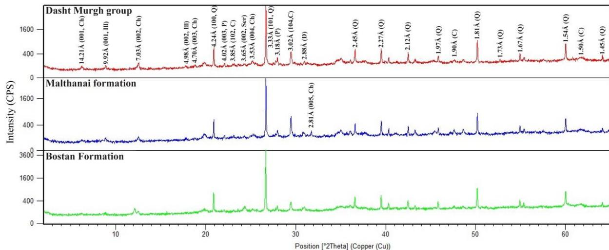
Fig. 4. X-Ray diffractograms showing 2θ and Å values of the relevant faces of various minerals identified in samples of the Dasht Murgh group, Malthanai formation and Bostan Formation in bulk mineralogical analyses. Abbreviations used: Ch = chlorite, Ill = illite, Q = quartz, P = plagioclase, C = calcite, Ser = serpentine, D = dolomite.
