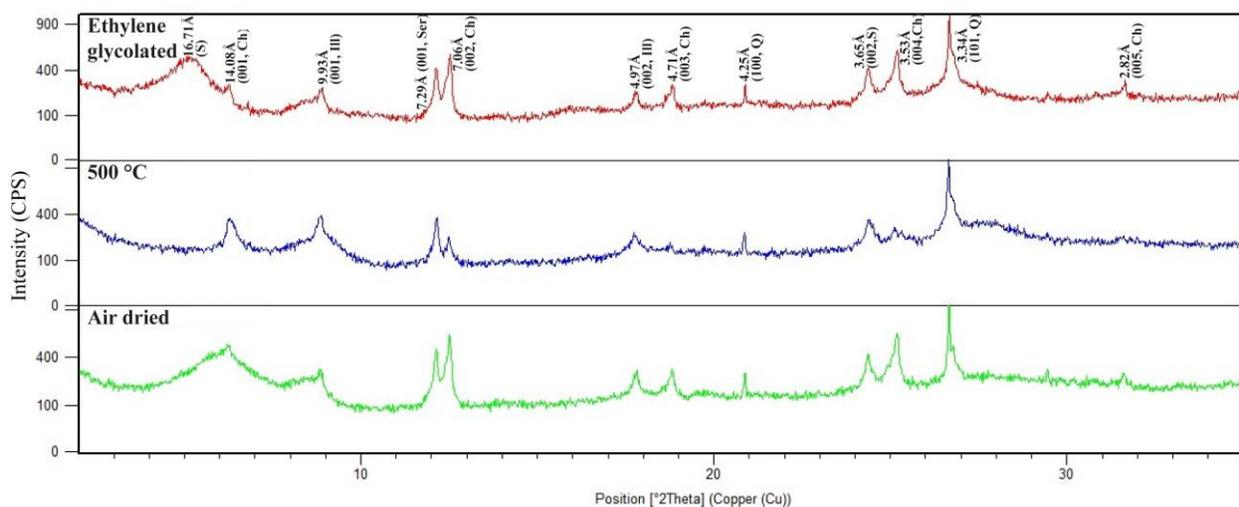
Fig. 7. XRD diffractogram of clay fraction of mudstone of the Bostan Formation, showing effects of different treatments on clay minerals.
