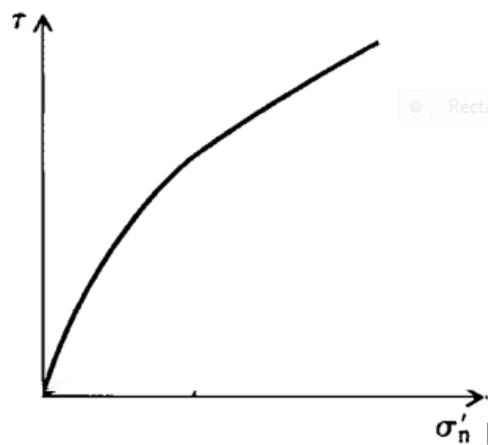
Fig. 2. Shear strength envelope for Barton model (after Barton and Choebey, 1977)
