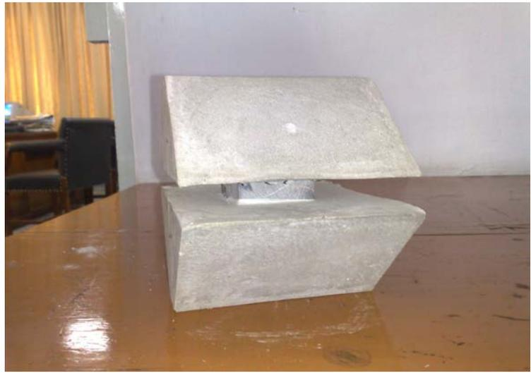
Fig. 3. Moulded sample for Shear box
