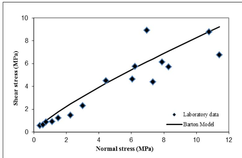
Fig. 4. Fitting of Barton model to Laboratory data.
