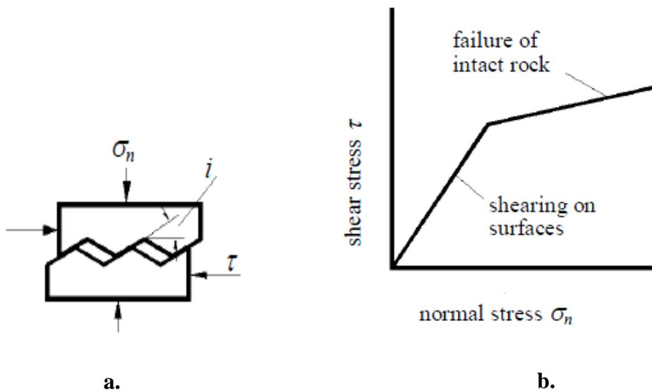
Fig. 1a. Shear Model for saw tooth surfaces, Fig. 1b) Shear strength envelope of Patton model (after Hoek et al., 1993)
