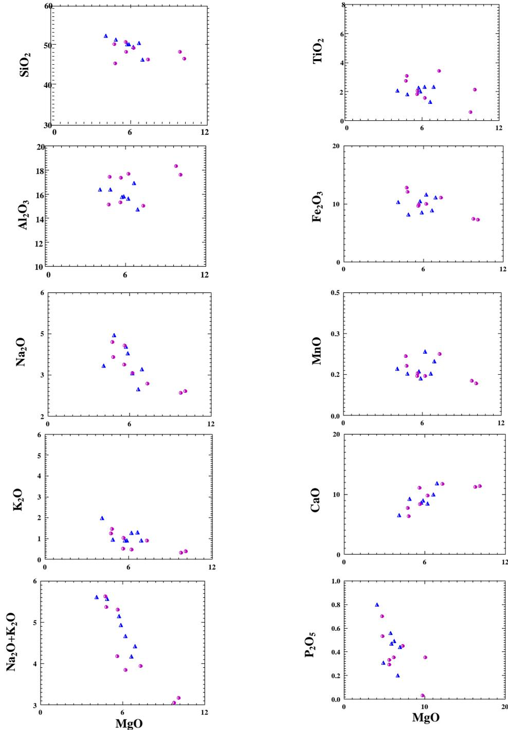
Fig. 7. Binary plots showing variation of major elements against  $MgO$  in the analyzed mafic dykes from Nagar Parkar.  $\blacktriangle$  Amphibole-bearing  $\bullet$  Pyroxene-bearing
