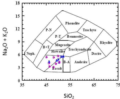
Fig. 4. Plots of the Nagar Parkar analyzed mafic dykes ( $\Delta$  Amphibole-bearing,  $\bullet$  Pyroxene-bearing) in the classification diagram of Cox et al. (1979). B-A: basaltic andesite; B+T: basanite and tephrite; Neph.: nephelinite; P-N: phonolitic nephelinite; P-T: phonolitic tephrite
