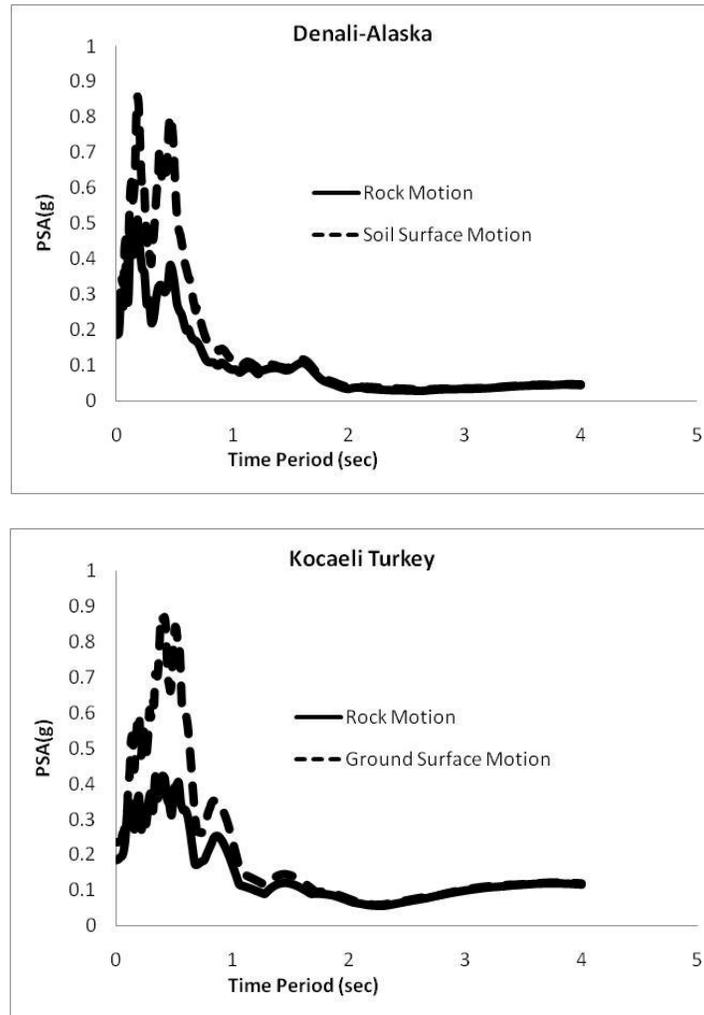
Fig. 11. Response spectra for soil and rock
