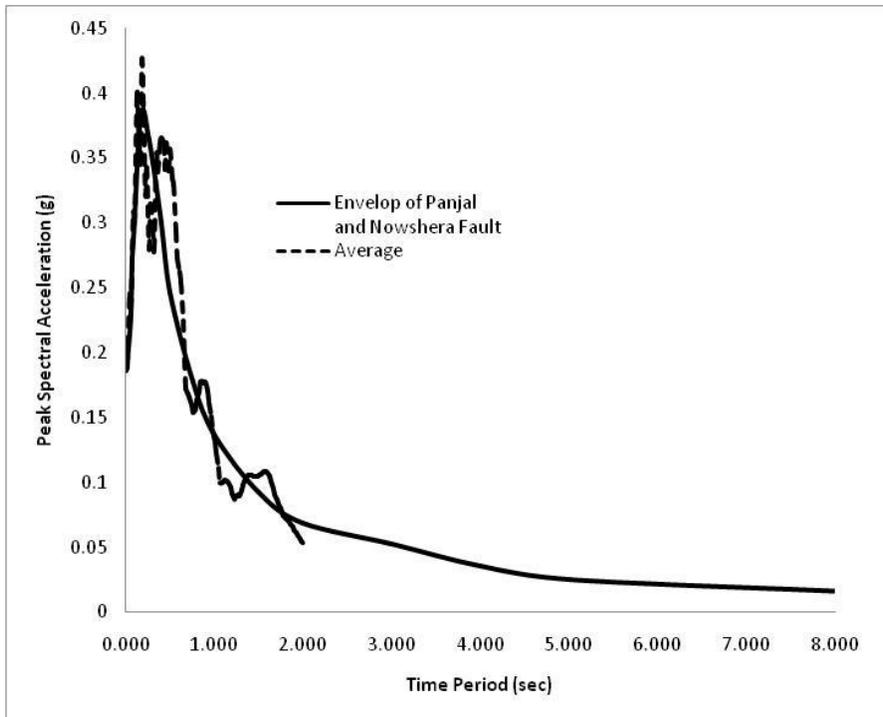
Fig. 9. Target response spectrum Vs average response spectrum
