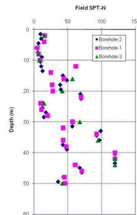
Fig. 1. Profile of Standard Penetration Test results
