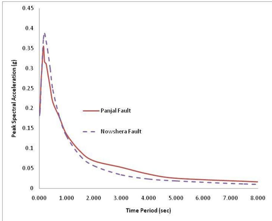
Fig. 5. Controlling response spectra at different periods
