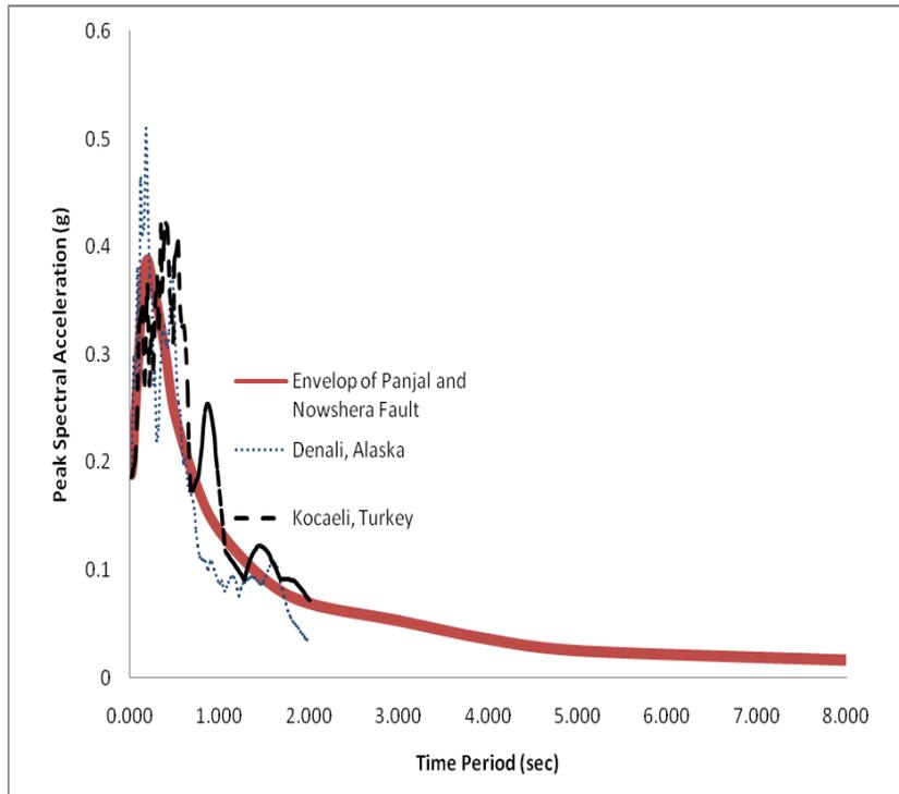
Fig. 8. Two scaled response spectra Vs design response spectrum
