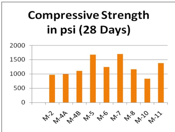
Fig. 8. Compressive strength of LWA
