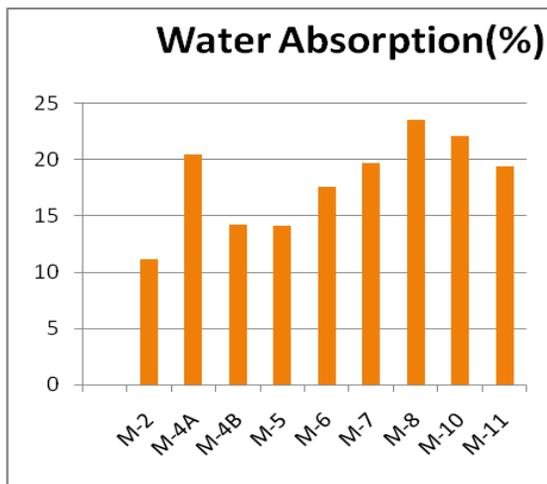
Fig. 2. Water absorption test of LWA
