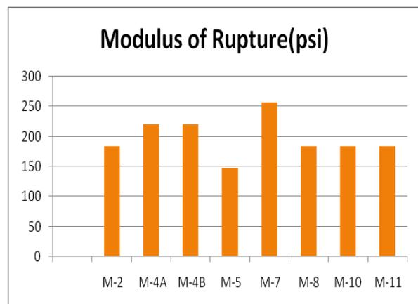
Fig. 9. Modulus of rupture LWA
