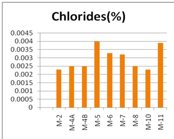
Fig. 6. Chloride content of LWA
