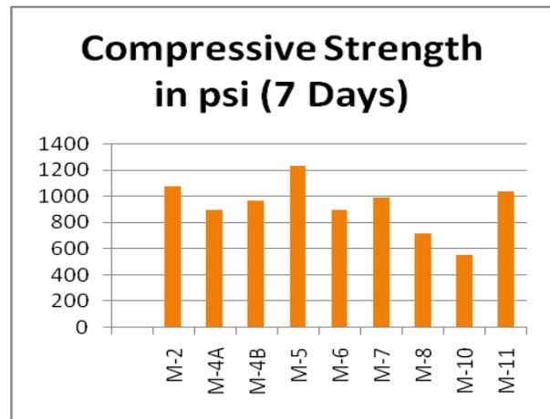
Fig. 7. Compressive strength of LWA
