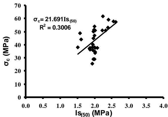
Fig. 3. Relationship between uniaxial compressive and Point load index for limestone from Kohat and Cherat
