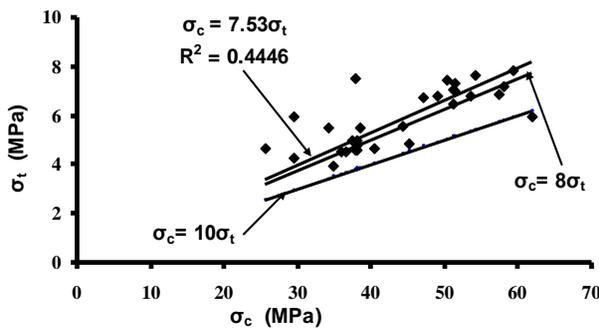
Fig. 2. Relationship between Compressive and Tensile strength for Kohat and Cherat limestones
