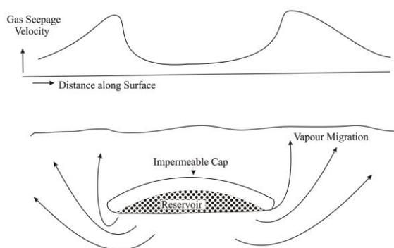
Fig. 2. Sketch of gas seepage from a simplified hydrocarbon Reservoir. The gas emission at the surface of the earth is indicated in the graph. “Reservoir” refers solely to hydrocarbons (modified after Zuhui et al., 1993).
