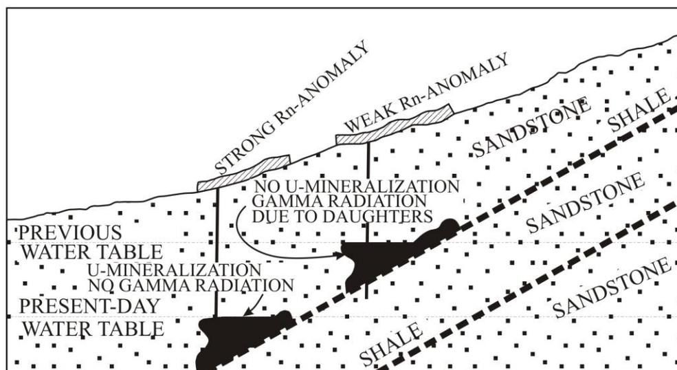
Fig. 1. The mobilization of uranium ore body detected by radon measurements using SSNTDs (after Qureshi et al., 1988).
