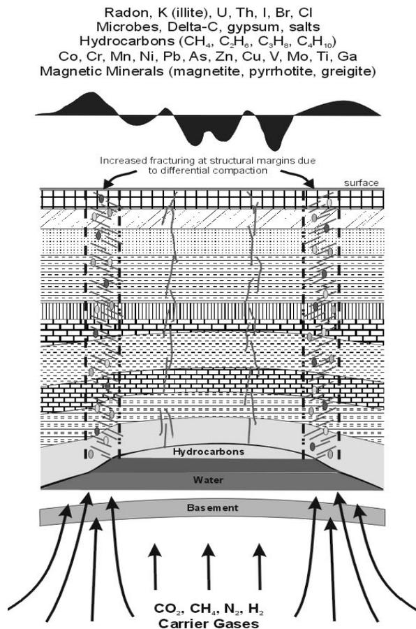
Fig. 3. The proposed working model for the formation of hydrocarbon, radiometric and geochemical anomalies at the earth's surface (after Sikka & Shives, 2001).
