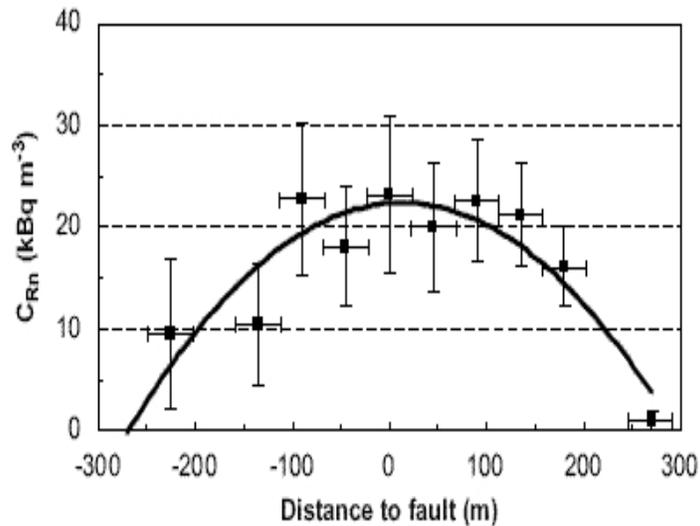
Fig. 6. Mean soil radon concentration versus the distance to the fault obtained with the LR-115 detectors in all transverse lines. The solid line is the second-order polynomial fit (after Font et al., 2008).
