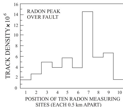
Fig. 4. Diagram showing radon peak over Main Boundary Thrust near Islamabad (after Qureshi et al., 1991).
