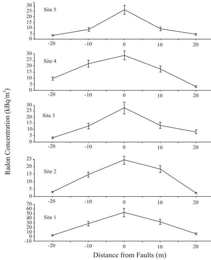
Fig. 5. Measured radon concentration values in soil gas from Jordan (after Al-Tamimi & Abumurad, 2001).
