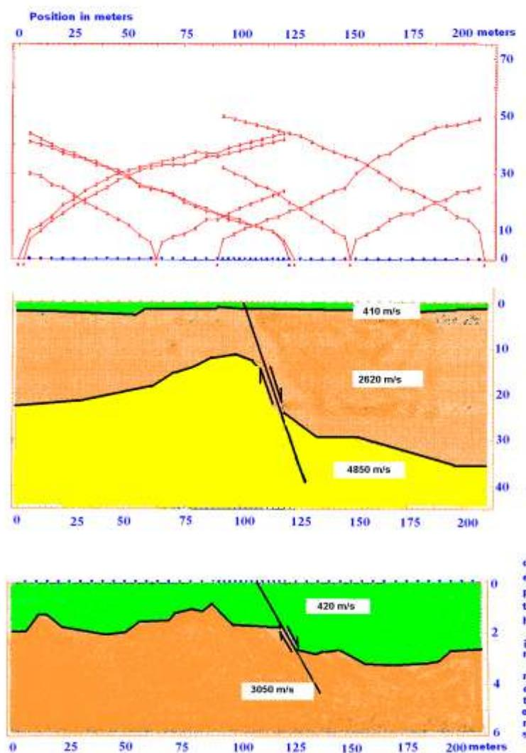
Fig. 4. Top: Composite T-X graph of seismic spreads A & B, parallel to the slide face.
