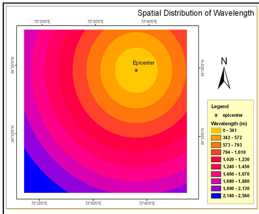
Fig. 5. Distribution of seismic waves wavelength during the 2005 Kashmir earthquake.
