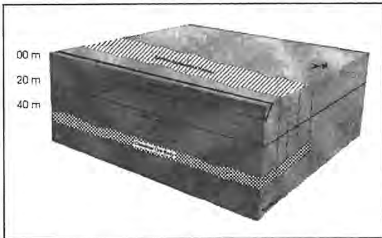
Fig. 4. Conceptual diagram depicting the mode of leaching of uranium from the surface out crop and corresponding accumulation in the sub surface below ground water table.
