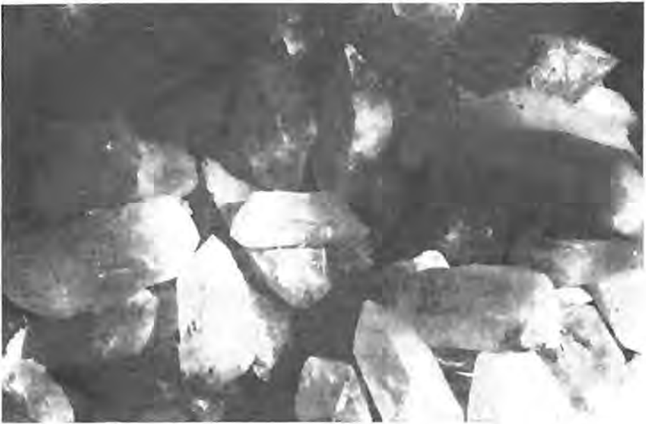
Plate 9. Lump of quartz crystals of various sizes collected from Shigar valley pegmatites.
