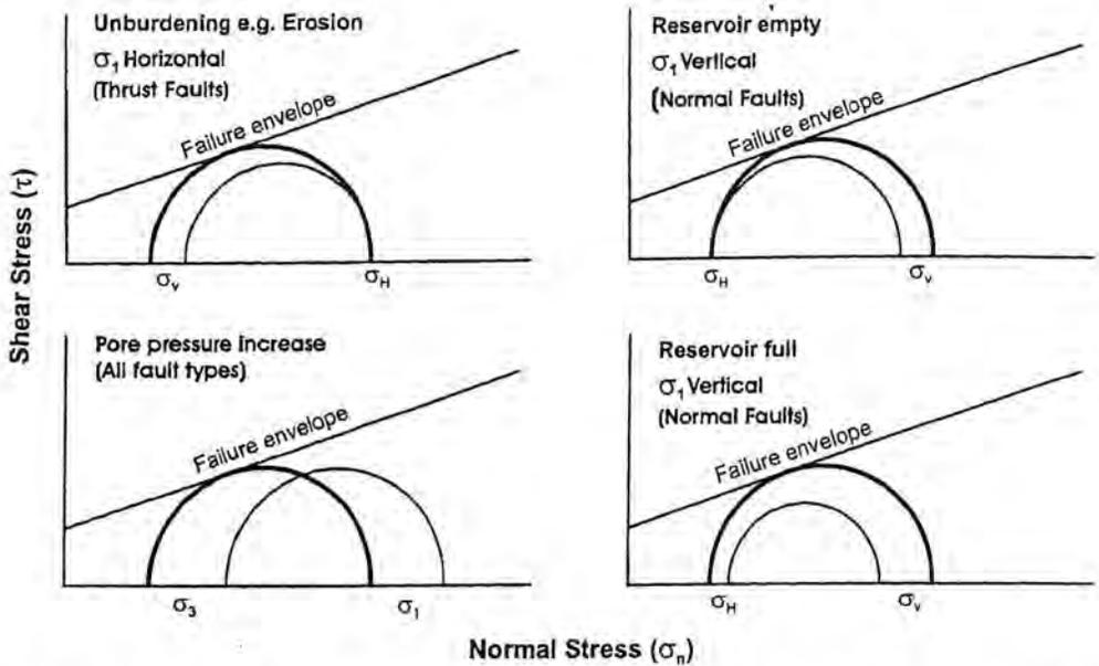
Fig. 5. Various environments in which change in stress leads to failure. Thick semicircle indicates the changed stress environment and thin semicircle denote original stress state. Intersection of semicircles with the failure envelope leads to failure.  $\sigma_H$  and  $\sigma_V$  refer to horizontal and vertical component of stress.
