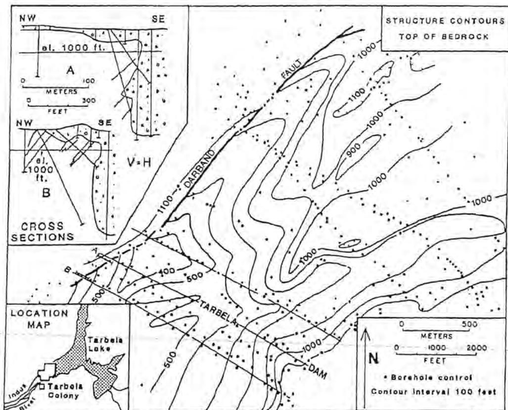
Fig. 5. Structure contours in feet of top of bedrock at Tarbela Dam. Darband fault marked by vertical to overhanging escarpment in bedrock, as noted in two cross sections. No vertical exaggeration in cross sections; scale of cross sections in larger than that of map.
