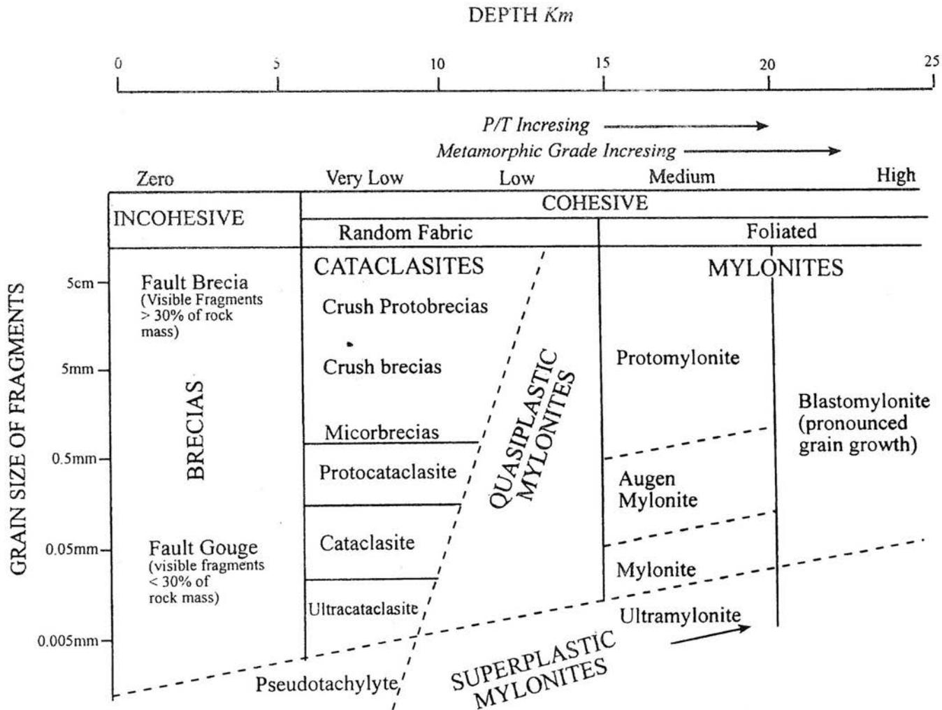
Fig. 2. Classification of fault rocks (Sibson, 1977).
