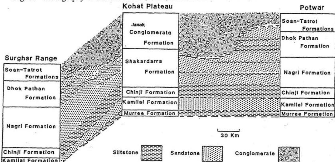
Fig. 4. Schematic stratigraphic sections of the Rawalpindi and Siwalik groups and equivalents from the Potwar area (east of Kohat Plateau), and the Surghar Range (south of Kohat Plateau). It shows large scale lateral lithological changes in the molasse sediments (after Gill, 1952; Meissner et al. 1974).
