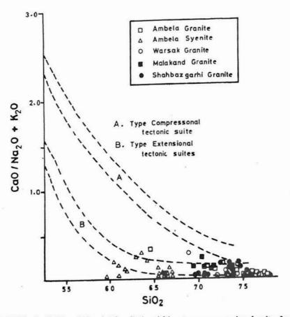
Fig. 5. CaO/(Na<sub>2</sub>O + K<sub>2</sub>O) vs SiO<sub>2</sub> plot for distinguishing type compressional suite from type extensional tectonic suites. Fields extrapolated from data compiled by Petro et al. (1980). The silicic rocks of the PAIP follow the trend of type extensional tectonic suites. Source of Data: Chaudhry & Shams (1983); Chaudhry et al. (1984), (1976); Hamidullah et al. (1986); Kempe (1973); Rafiq & Jan (1989).
