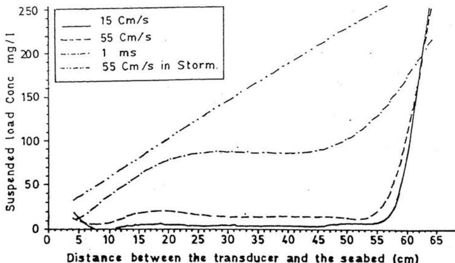
Fig. 6. The distribution of particles in the water column for various tidal current velocities. At low velocities the particle size is fine and uniformly distributed but as the coarser fraction of the bed sediments start to move at higher velocities the water becomes stratified.
