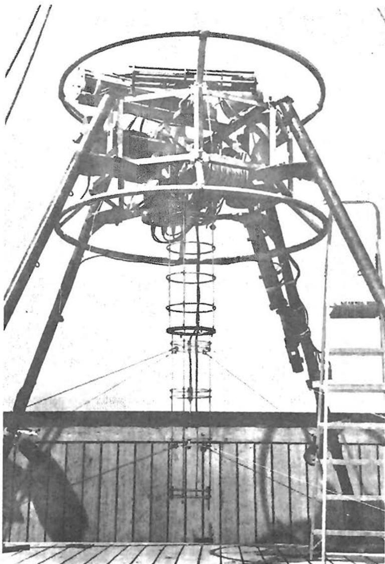
Fig. 1. MAFF tetrapod equipped with the ABM, electromagnetic current meters, optical transmissometer, and other instruments ready for deployment.
