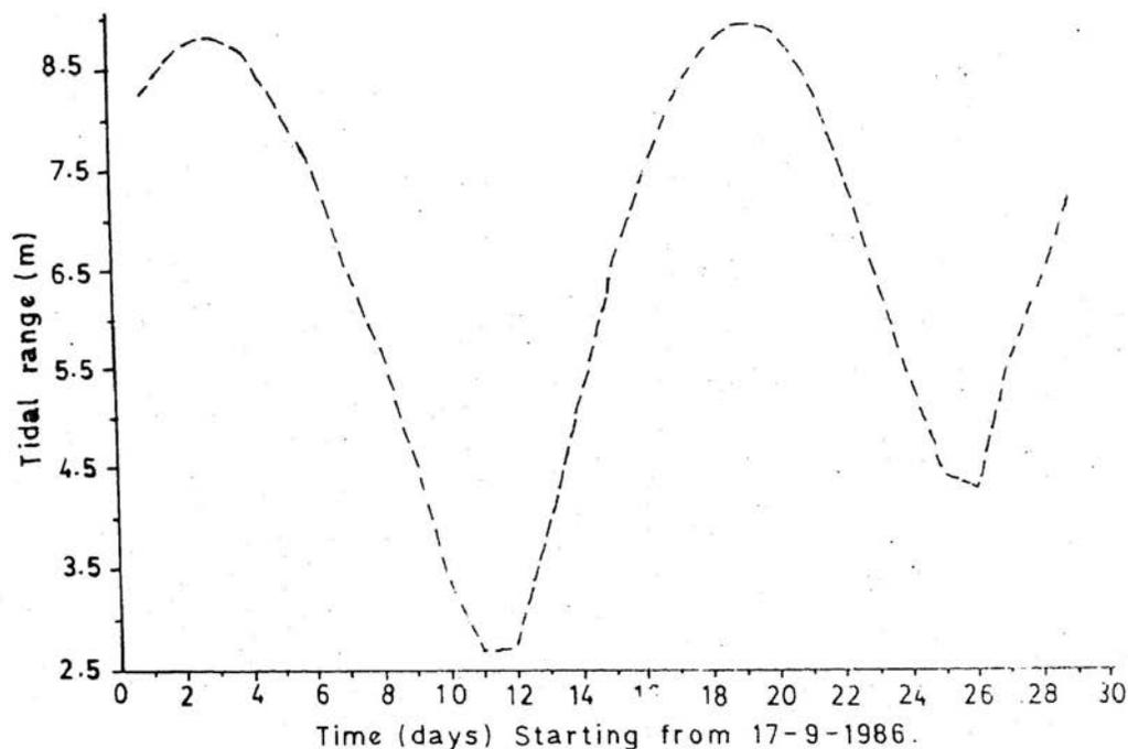
Fig. 4. The tidal range (m) for Liverpool Bay area corresponding to the time of ABM deployments at stations A and B, respectively. Mean daily range from (a) 17-7-1986 to 15-8-1986. (b) from 17-9-1986 to 16-10-1986.
