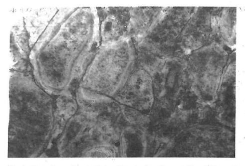
Fig. 4. Photomicrography of elliptic pellets showing allignment (Plane Light, x 25).
