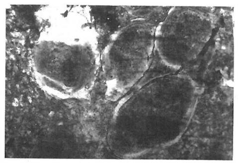
Fig. 3. Photomicrography showing uniform distribution of oval shaped pellets (Plane Light, x 25).
